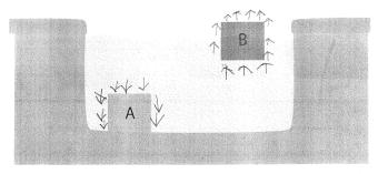
Block **A** has sunk in the water and Block **B** is floating. Can you draw upward arrows **1** and downward arrows **1** on this illustration to explain why the blocks behaved the way that they did?
