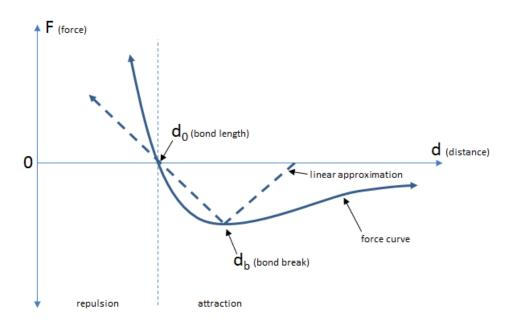
The main features of the force curve are maintained: a repulsive force when the distance d is less than the bond length  $d_0$ , an attractive force when d is greater than  $d_0$ , and a falling off of the attractive force past a given distance  $d_b$  where the bond "breaks." The advantages of the
